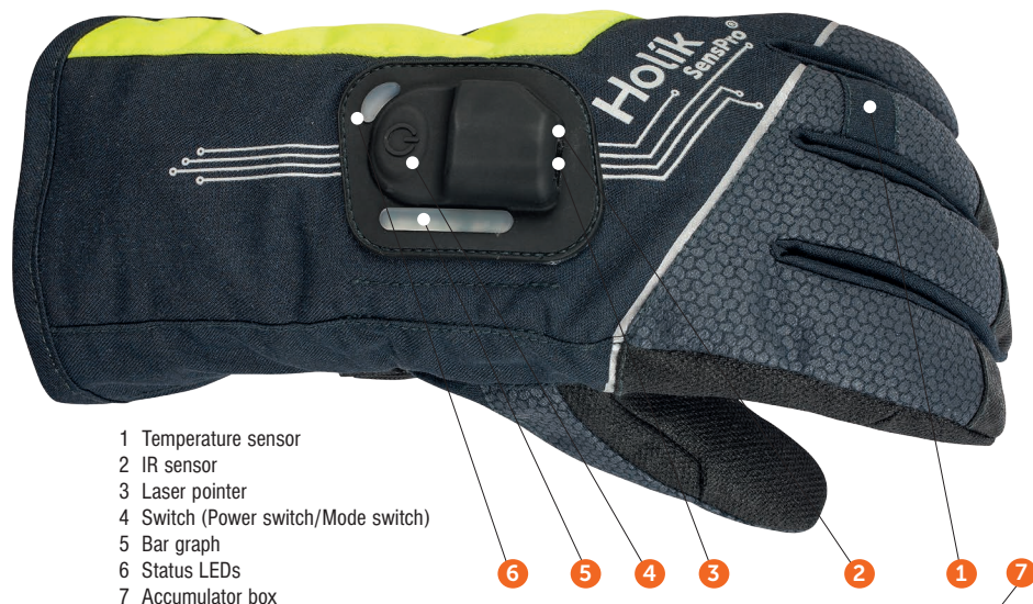
Fig. 1: Location of functional elements on the back of the glove
